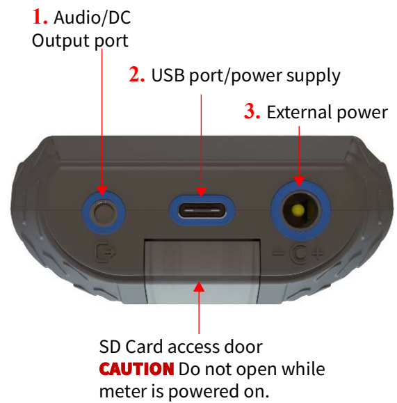
Figure 1-2 Main Body: Bottom Connectors
