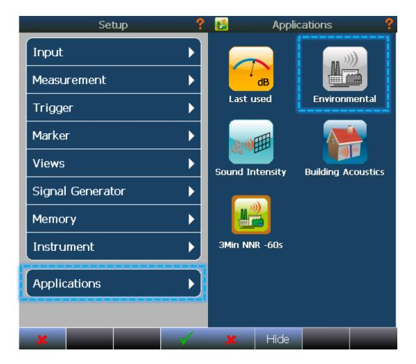
Press SETUP Key to start adjusting your settings for noise nuisance settings
